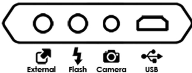
The camera cable port is a 2.5 mm stereo female jack. The camera cables have the male 2.5 mm stereo jack on one end. This end is plugged into the camera connection port. The other end changes depending on the camera make and model. This end is plugged in the shutter release port of your camera.
