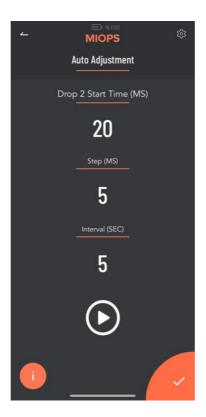
Drop Start Time (MS): This is inital drop size value for Auto Adjustment Step (MS): Drop Size increment value on each iteration Interval (SEC): The interval value between each iteration
