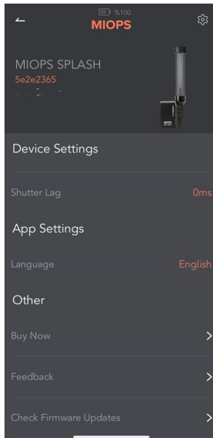
If your device has the latest firmware version, you will see a message on the screen like "Your device is up to date". If there is an available firmware version, you can start the upgrade process using this screen.
