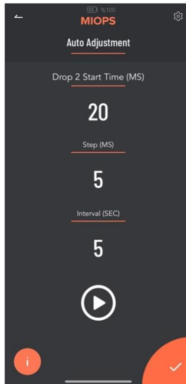
**Drop Start Time (MS):** This is initial drop size value for Auto Adjustment
